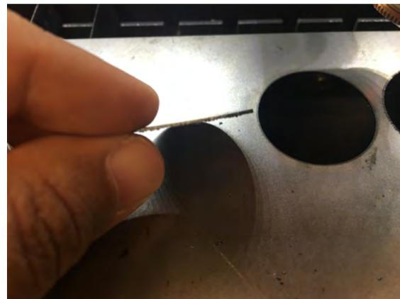
Now if you notice any burring at the bottom of your metal piece and you've already tested different PSI levels of oxygen, you may need to change your **Follow Height** (moving the focal point) to help reduce the amount of burring.
