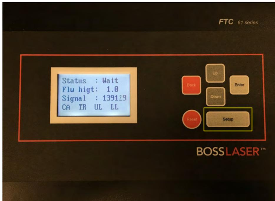
Now move the laser head's nozzle by using the **Up and Down buttons from the FTC 61 Series Control Panel** very close to the material, but not touching (about 5mm gap), as illustrated in the picture showing the metal head w/ the metal sheet.
