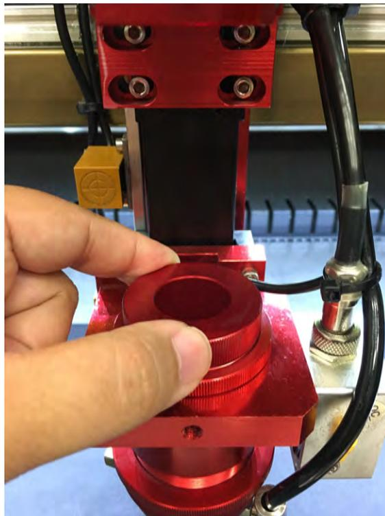
**For the Metal Head, there is a separate piece for the lens housing (shown above; being held by the hand in the picture)**
