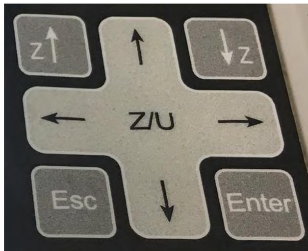
Now that you have the Metal head calibrated and above your material, position the laser head to be on the top-right of your work area (this area is where you want your cut out to be). The reason behind being at the top-right is because, by default, the origin point is set to the top right of the cut out.
