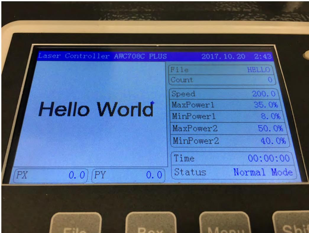
Using the **Directional Arrow buttons** (shown below), move the laser head above your material, for this exercise, a piece of wood (birch wood).
