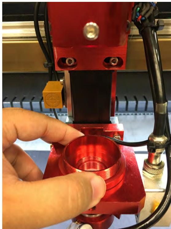
Now installing the Metal head is the same way you would install the Non-Metal head (held by a retaining nut), but you'll need to make sure you install the **Blue Signal Cable** to the **Amplifier (Silver Box)**. Also, make sure you have installed back the 6mm hosing to the nozzle (as shown below):
