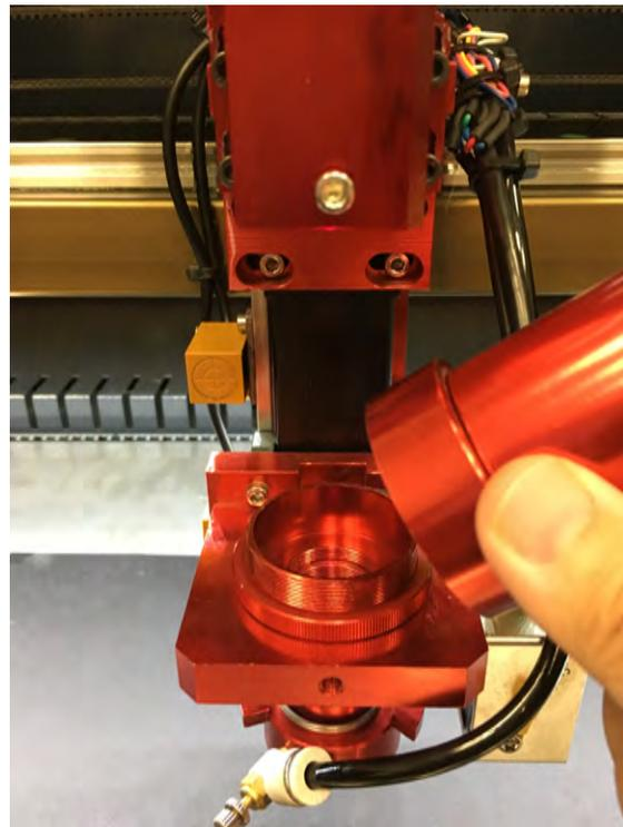
As shown below, loosen the retaining nut that is holding the **Non-Metal lens housing** and remove it from the laser head assembly. You'll need to unhook the 6mm hosing from the nozzle to complete remove the lens housing.
