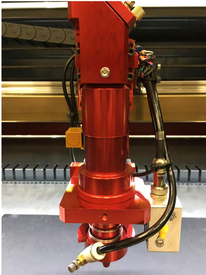
Now rotate the set screw to unlock and drop the dust cover out from the laser head assembly (as illustrated below):
