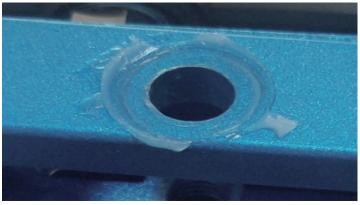
b. Apply grease to the head of the thread and the bottom surface of the black part, as shown in the red part, and then reinstall it, the situation will improve a lot
