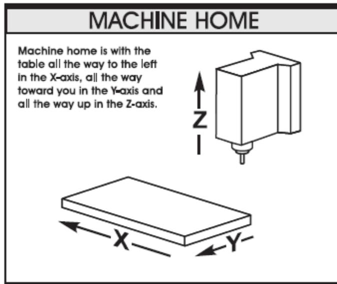
This is crucial to the operation and function of a CNC machine as all of our programs, fixtures, and tooling are based off of the **machine home position described as X0, Y0, Z0.**
