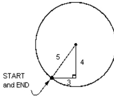
To cut a complete circle of 360 degrees (360°), you do not need to specify an ending point **X**, **Y**, or **Z**; just program **I**, **J**, or **K** to define the center of the circle. The following line will cut a complete circle:
