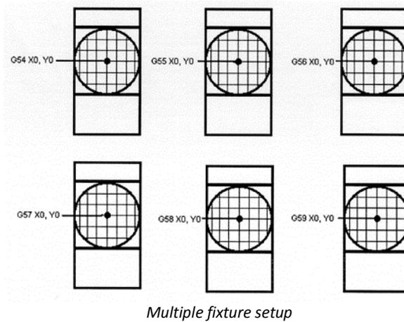
The figure above represents a multiple-fixture setup. Each vise will have an absolute zero once it is specified in the program. This is done by using G54 through G59. G54 through G59 and G154 P1 through G154 P99 gives a total of 105 different work offsets which may be used.
