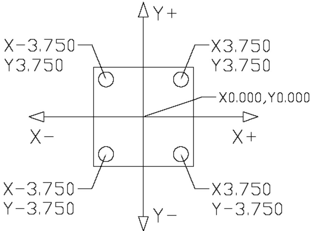
Vertical machining centers have 3 axis of travel. We have talked about two of them, the X (left to right movement), the Y (moving the part towards and away from the operator), but the last to discuss is the Z. The Z axis moves the milling spindle up or away from the part in the positive direction, and towards or into the part in the negative direction. Now that we have discussed all 3 of the axis, we can take a look at this picture of a Haas VF-8 VMC.
