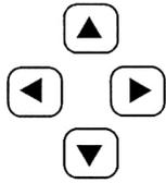
**Cursor Keys** The cursor keys are in the center of the control panel. They give the user the ability to move to and through various screens and fields in the control. They are used extensively for editing and searching CNC programs. They may be arrows or commands.
