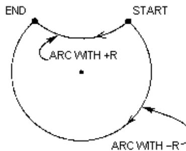
The following line will cut an arc less than 180 degrees (180°):
