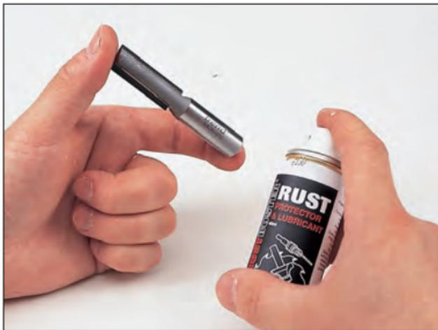
Before storing your cutters, apply an anti-corrosion spray such as Rustbuster®. This is particularly important if the cutters will be stored in humid conditions, such as in a shed or workshop, that suffers from excessive changes in temperature. This will prevent surface corrosion forming that will cause the cutter to bind in the collet. Be sure to keep spray away from the ball-bearing guide.
