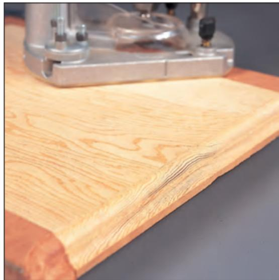
When trimming or moulding only across the grain (i.e. leaving the long grain edges square), speck battens can be clamped at the ends of the panel to prevent break-out.
