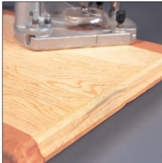
When trimming or moulding only across the grain (i.e. leaving the long grain edges square), spelch battens can be clamped at the ends of the panel to prevent break-out.
