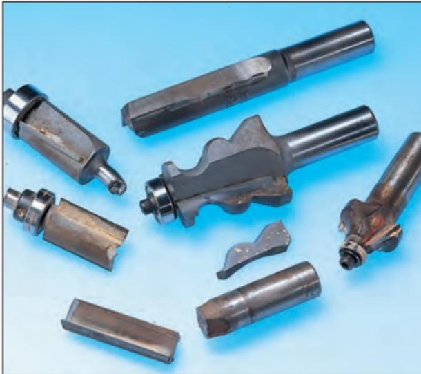
Although the structural and metallurgical composition of components that are used in the construction of a quality router cutter are designed to withstand professional and industrial use, damage or breakage can and does occur for many reasons. A detailed examination and statistical analysis indicates three distinct causes.
