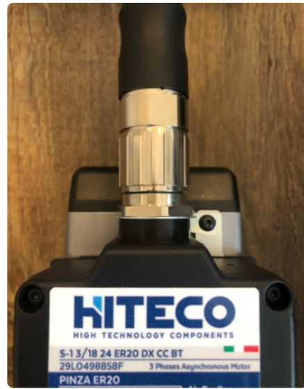
M23 Cable Tightened
